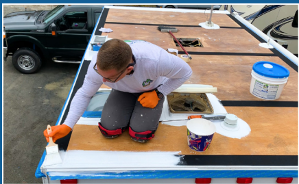
CUT-IN WITH CRAZY SEAL TO PREPARE FOR ROLLING
