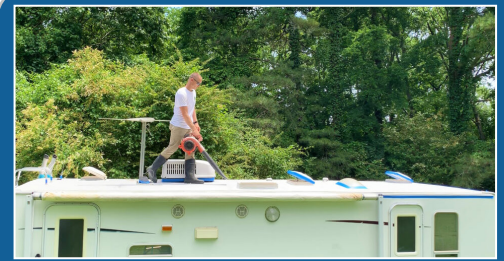
REMOVE DRY PARTICLES WITH A LEAF BLOWER
