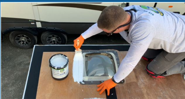
APPLY A THICK AMOUNT OF CRAZY PATCH OVER ALL PENETRATIONS LIKE AROUND SKYLIGHTS
