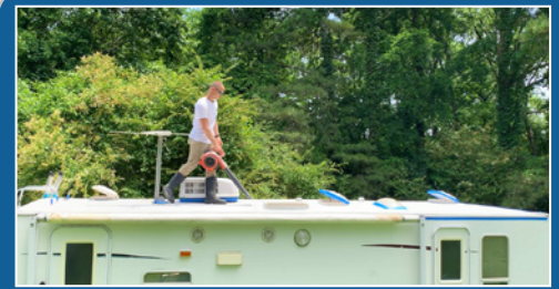
REMOVE DRY PARTICLES WITH A LEAF BLOWER
